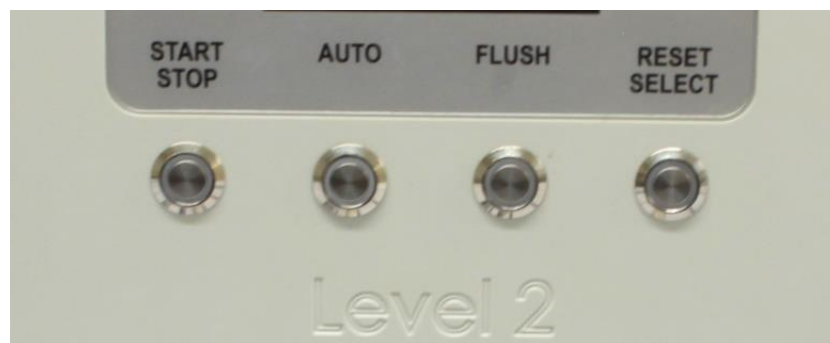
Figure 26: Operator Control Panel (OCP) Button Detail
