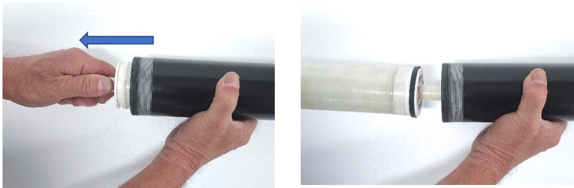
Figure 32: Pulling the Membrane Element Out
