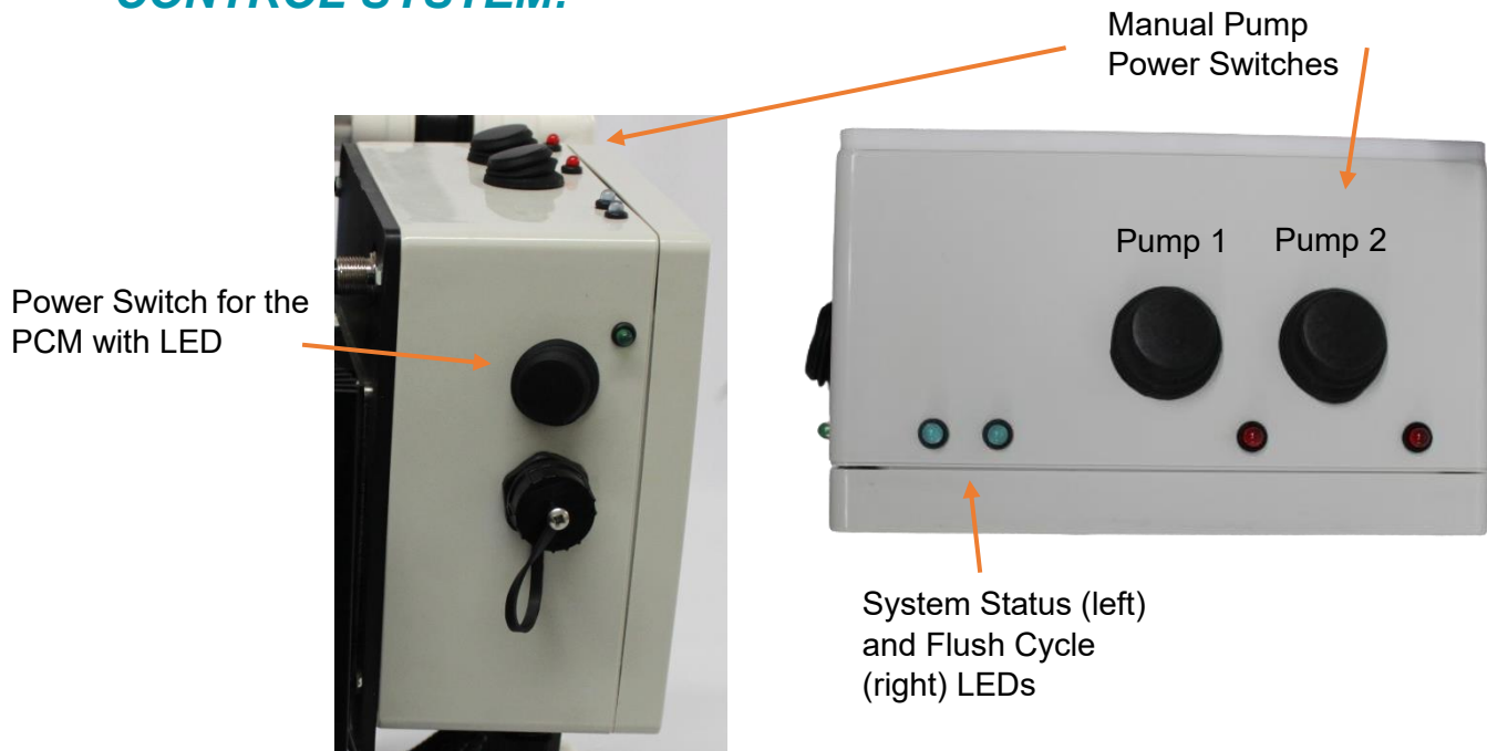
Figure 25: Pump Control Module (PCM)
