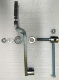
2.Exploded view of tensioning arm components – Note aluminum space between pin and arm may not be required.
