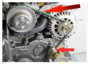
1. First remove bolt(s) securing the original tensioning arm and the cover support bolt illustrated above.
