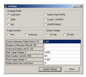
The tachometer output is dependent upon the correct crankshaft pulley to alternator pulley ratio being defined, as well as, the number of alternator poles.
