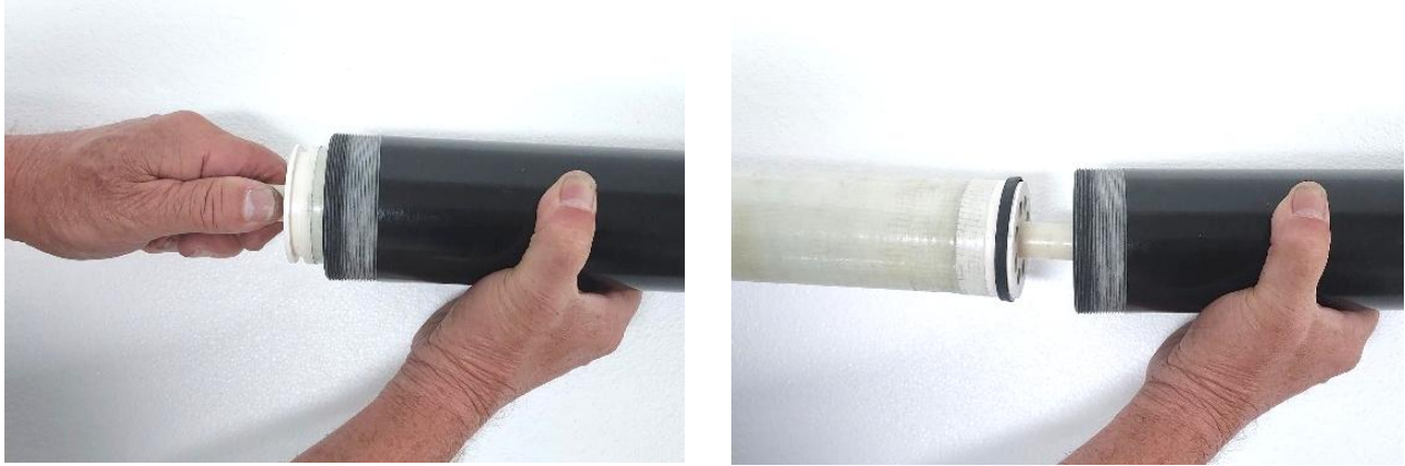
Figure 32: Pulling the Membrane Element Out
