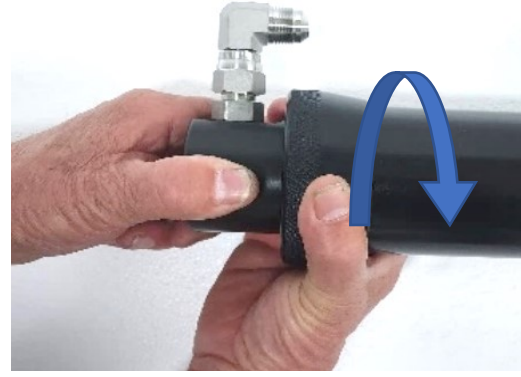
4-Finish threading the Ring on and hand tighten just snug
