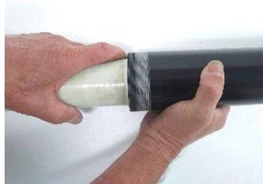
4-Align the Membrane with the Tube and push the rest of the way in
