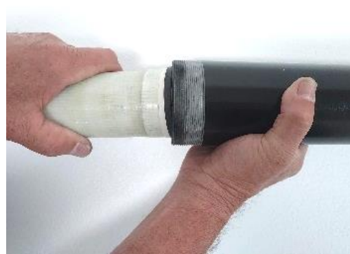
2-Place Seal into the Tube at an angle
