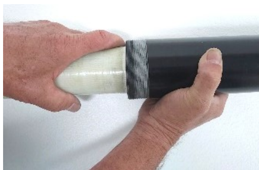
4-Align the Membrane with the Tube and push the rest of the way in
