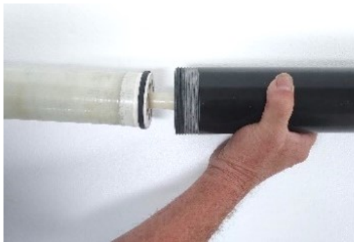
1-Insert Membrane into the Outlet end of the Pressure Vessel Tube
