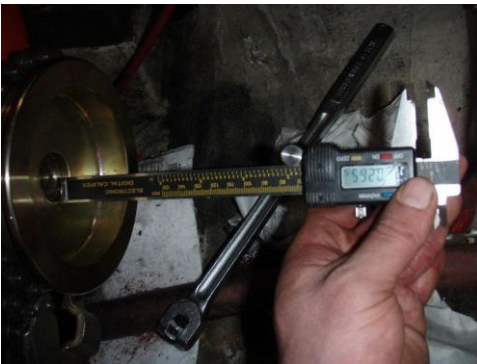
7. Even after it has been pressed on and tightened down, you will have a 1/4" space from the end of the shaft to the face of the pulley. (a note on chain grips like the one wrapped around the pulley here.. Use a piece of leather or something similar to wrap the pulley first so that the ribs of the pulley do not get dinged up.)
