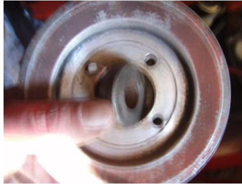
5. You will need to reuse the washer from the original pulley so that your bolt can hold the new pulley in place better.
