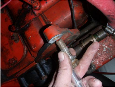
16. Using new mounting bolt and spacer bushing supplied with the Aquamaax alternator
