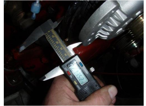
18. After installing the alternator with the mounting spacer, you will need to use the other tensioning bracket spacer and bolt provided to tighten the belt
