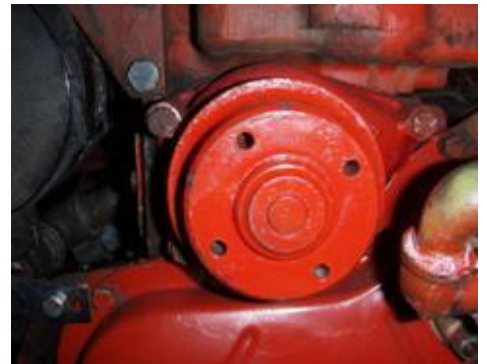
9. Remove Old Water Pump
