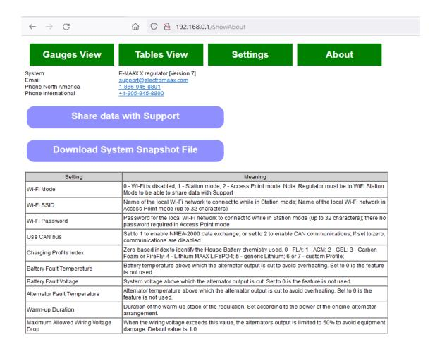
Shown above is the "About" page which allows connection to ElectroMaax Technical Support; if support is not available the system information can be saved as a Snapshot file that can be sent to technical support for review. The snapshot shows system state values at the instant it is created. You can view the Snapshot from the web interface by dragging/dropping the file onto the Windows software.
