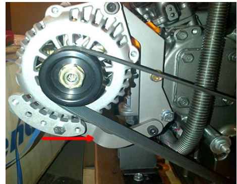
6. Connect adjustment arm to Bolts provided in kit.
