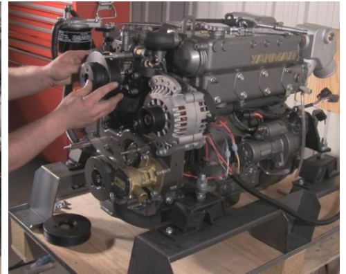
3. Bolt on water pump pulley with 4 bolts supplied in kit
