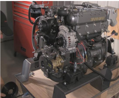
4. Water pump pulley installed
