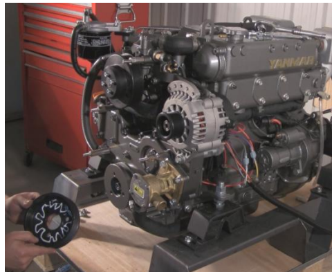
5. Apply barrier tef gel to inside of the crank pulley shive
