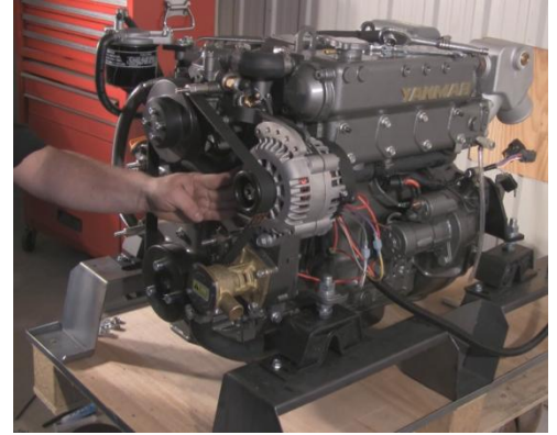
9. Tighten bolt on tensioning arm
