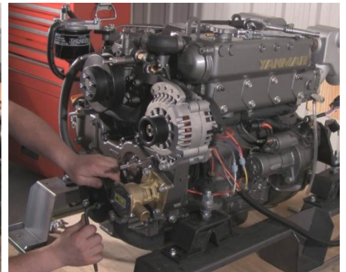
6. Mount crank pulley over existing crank pulley attach with bolts
